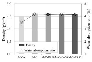
Fig. 5 – Density and water absorption ratio of each coarse aggregate
