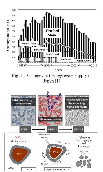
Fig. 2 – Improvement of concrete strength by modification and recovery by microwave heating [8,13]
