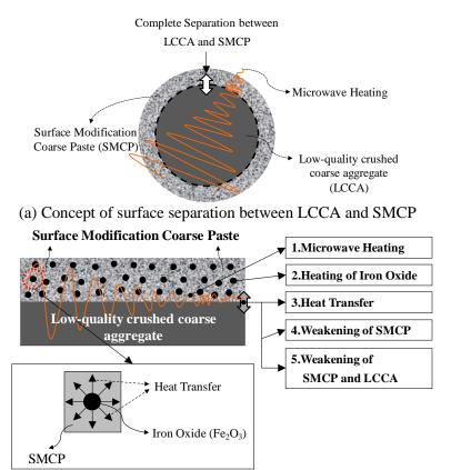
(b) Control factor of surface separation of modification aggregate Fig. 4 – Mechanism of weakening between LCCA and SMCP [7-9]
