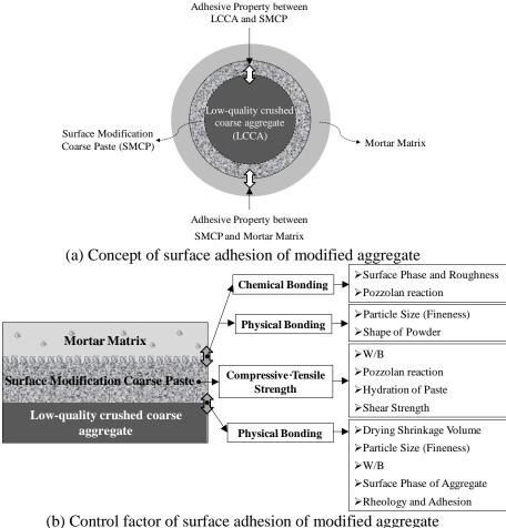
Fig. 3 – Mechanism of adhesion between modified aggregate and interface [7,8]
